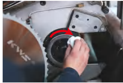
2 Flange must be free from scratches and wiped clean.
