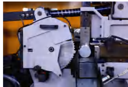
5 The length of work piece should not be shorter than 20mm. Otherwise, the saw blade will be broken.
